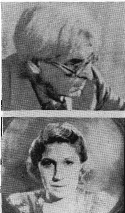
Fig. 6. (Top to bottom, a, b, c, d, e) Various television images taken with interference at a frequency of about 300 kc. Interference to signal voltage ratios: 0, -10, -20, -30, -40 db.
